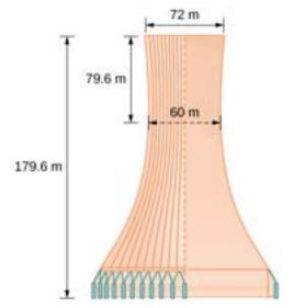
Figure 11 Project design for a natural draft cooling tower
